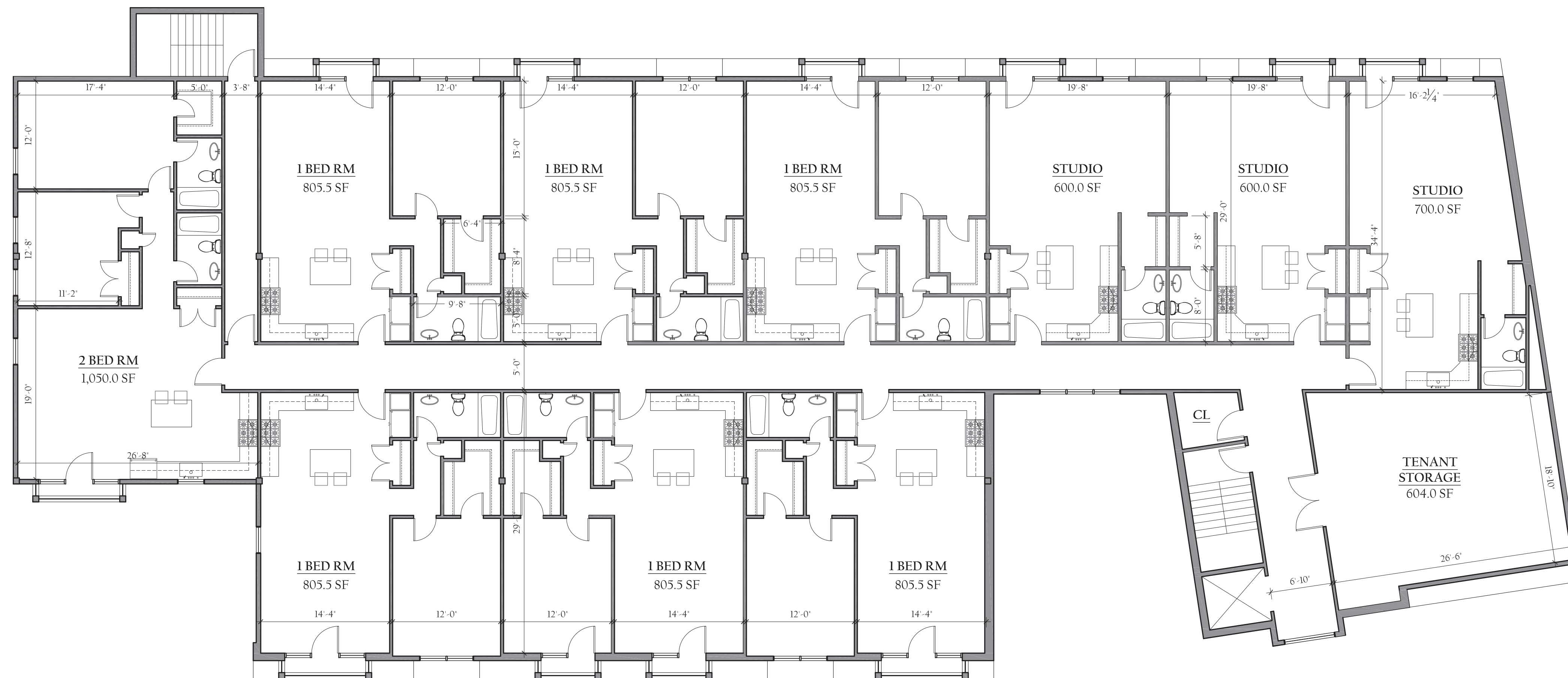
2 PROPOSED 4TH FLOOR PLAN A-1 SCALE: 1/8"=1'-0" TOTAL BUILDING AREA 4TH FLR: 9,771 SF
