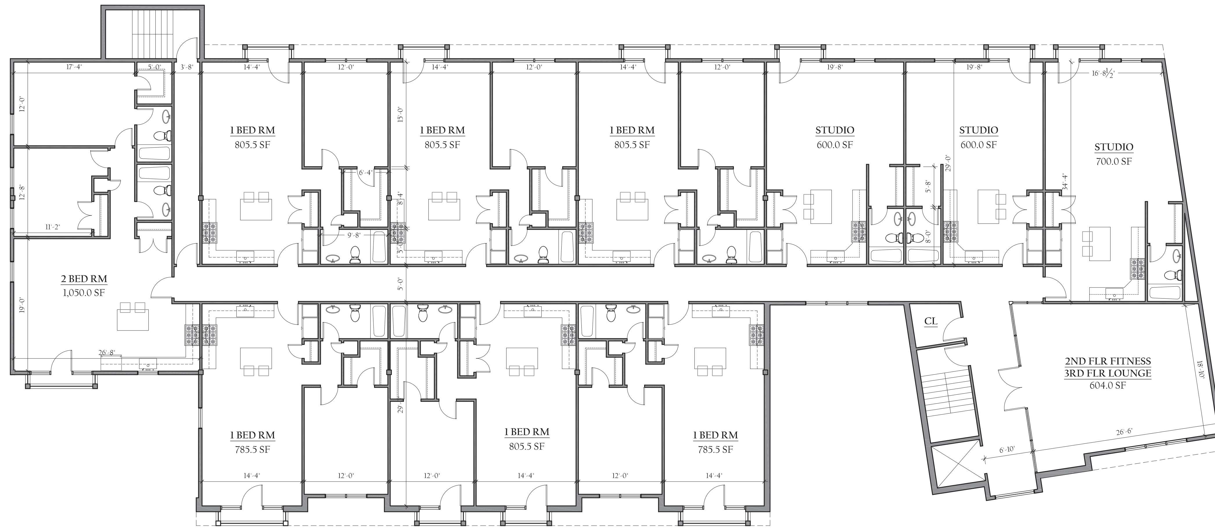
1 PROPOSED 2ND & 3RD FLOOR PLANS A-1 SCALE: 1/8"=1'-0" TOTAL BUILDING AREA EACH FLOOR: 9,727.0 SF
